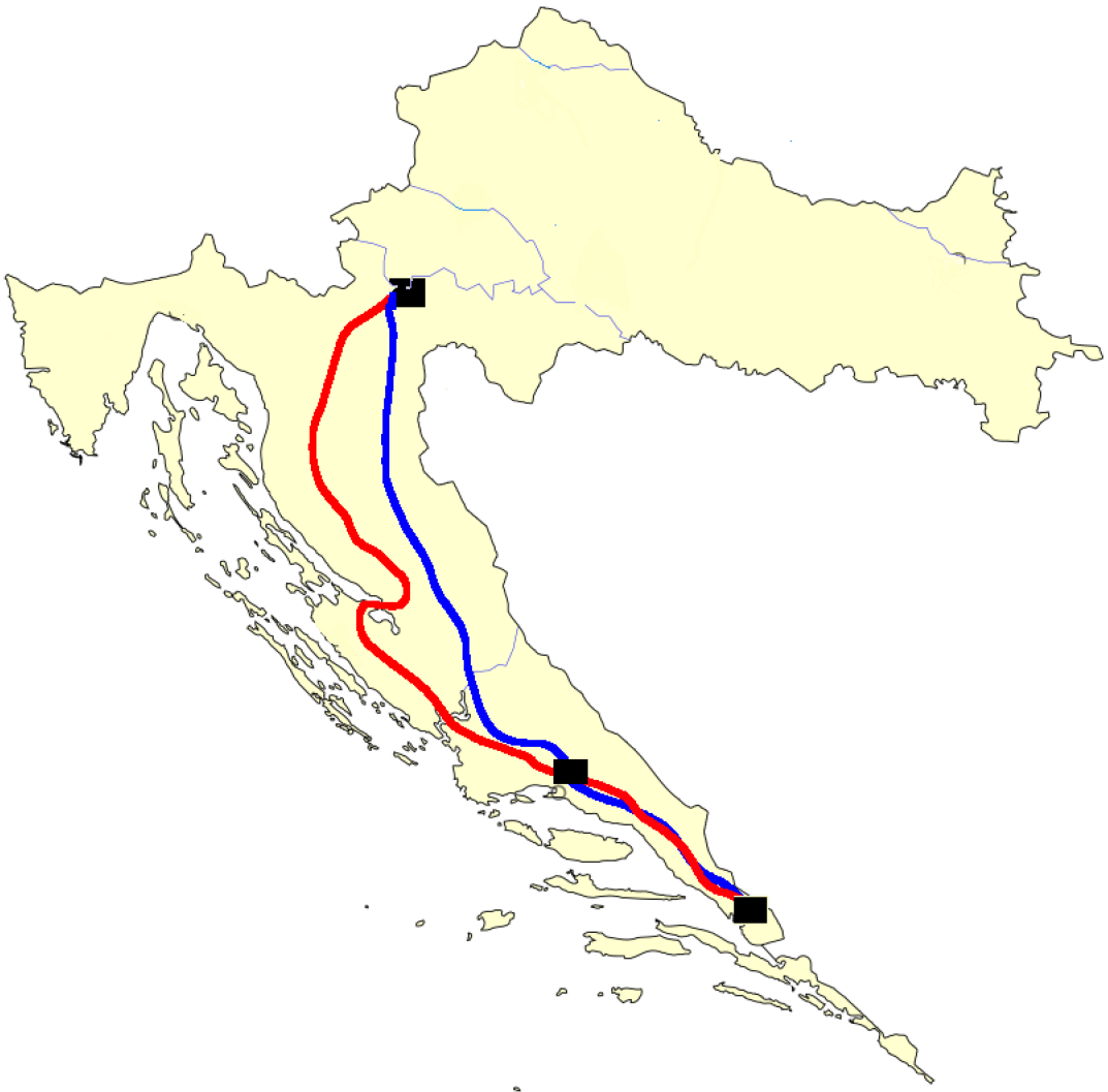
FIGURE 2 Actual A1 highway and terrain-based LCP. Notes: Approximate map of the actual A1 highway (in red) and the LCP (in blue). The black dots represent the nodal cities of Karlovac (in the north), Split, and Metković (in the south).
